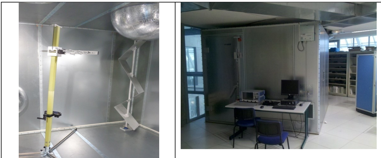
Reverberation chamber: ETS-LINDGREN +VNA R&S ZNB8 8GHz+SA HP8591E 26 GHz
