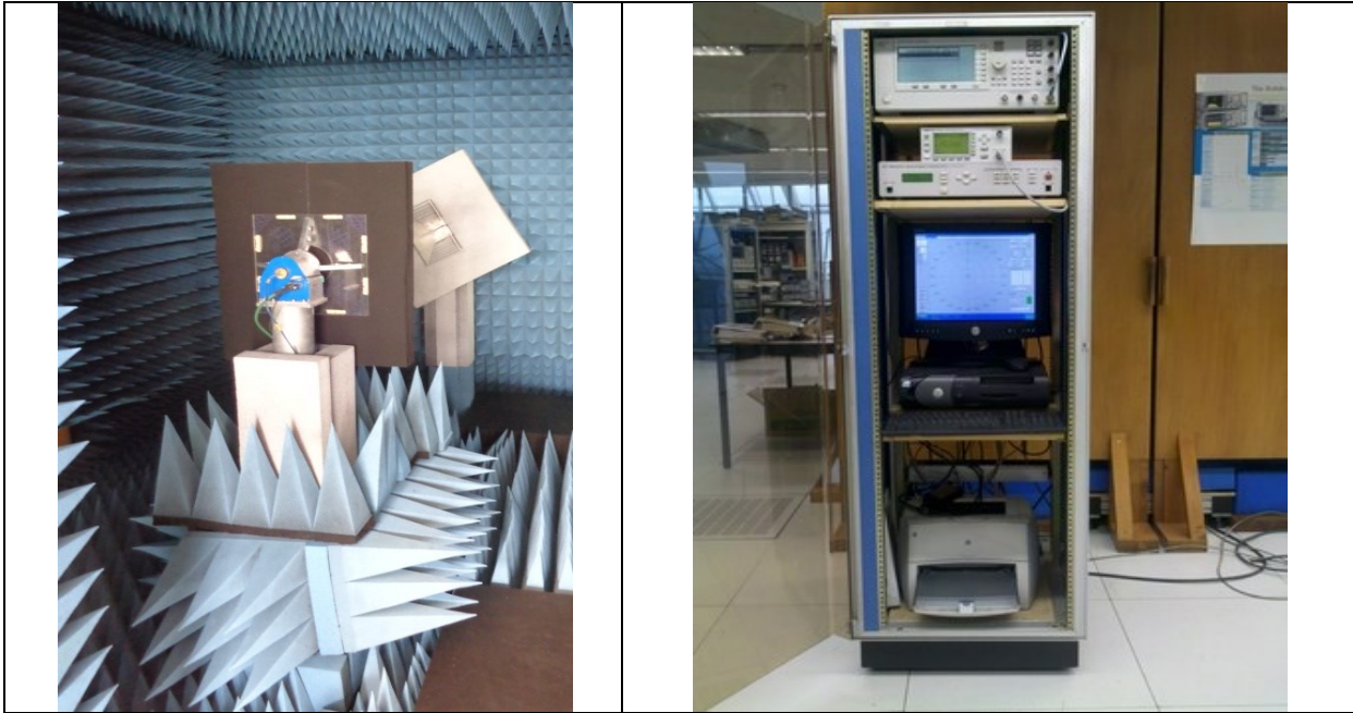
Anechoic chamber: ASYSOL Anechoic chamber (Near field measurement) 800MHz – 40 GHz +VNA HP8720B.
