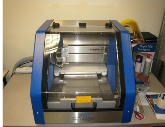
Mechanical engraving machine: Protomat LPKF S100 CAD-steered milling technology established as an efficient and pollution free alternative to chemical etching for the fabrication of printed circuits (antennas or RF circuits)
