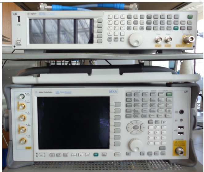
Vector Signal generator N5182A 6GHz + Signal analyzer 9020A
