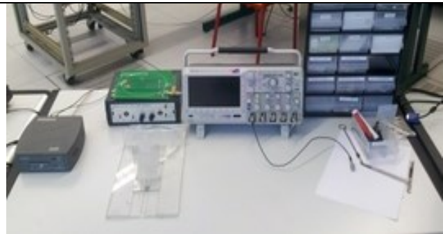
HF RFID tag measurement setup at 13.56 MHz
